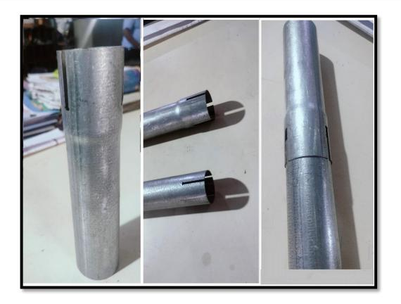
Ram forming swaging machine--pipe reduction Tool- Gripper, insert, finger type tooling(sizing ratio 5mm).
