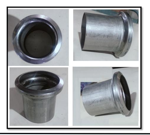
**Rolling(beading) Machine Operation Component.**
