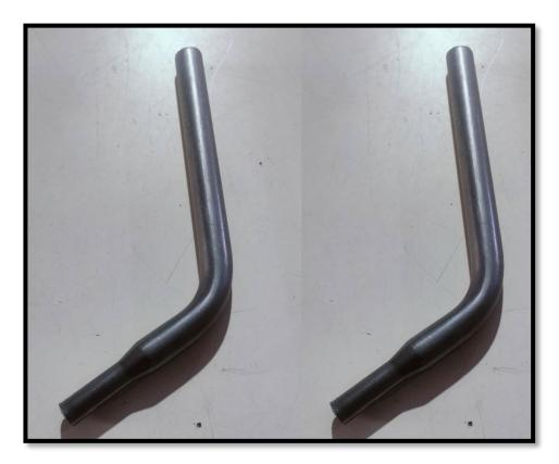
Pipe OD Ø12.65mm After sizing Pipe OD Ø9mm Sizing length 24mm.
