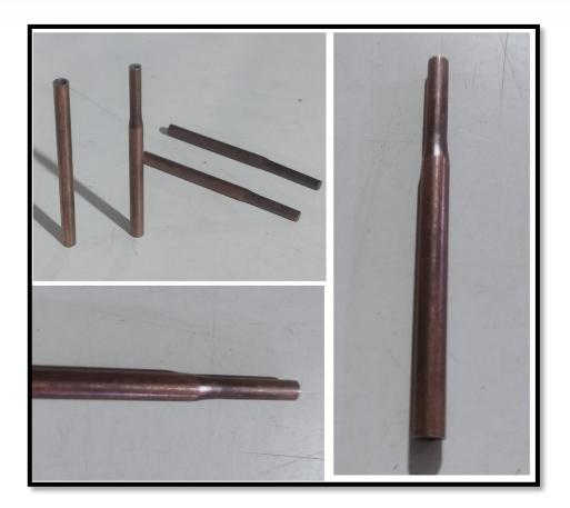
Auto feeding Rotary swaging Machine(Hammering pipe Operation)
